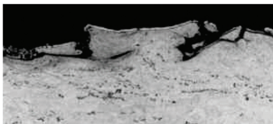
Damaged Surface from Broken Media
