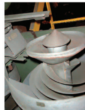
Figure 15 Spiral Separation System for Shot Media Classification
